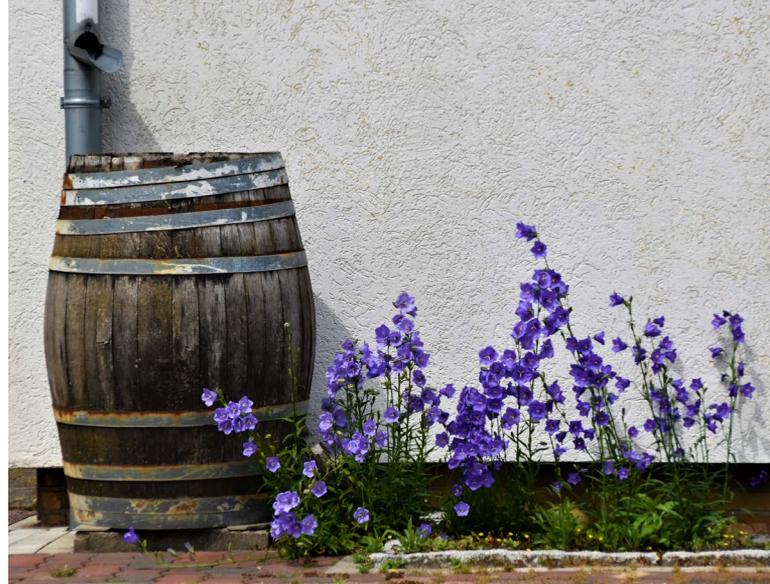
The simplest way to install a rain barrel is positioning a plastic or wooden barrel directly under your gutter downspout. Basic piping may be required, but this is an easy way to harvest rainwater, and the barrel won't take up much space. Consider a cover for the top of your rain barrel to keep insects and small debris out of your harvested water.
